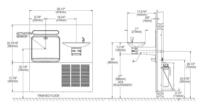
NOTE: New Installations Must Use Ground Fault Circuit Interrupter (GFCI). It is highly recommended that the circuit be dedicated and the load protection be sized for 20 amps.
